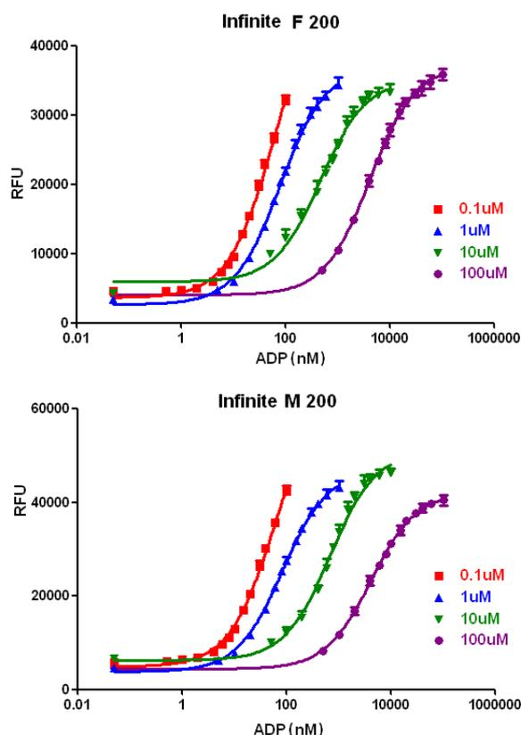
**Figure 2:** Sample data for 0.1 μM, 1 μM, 10 μM, and 100 μM ADP/ATP standard curves generated with a flash number of 100 for both instruments.
