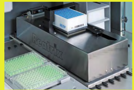
The REMP Reatrix 2D Scanner can be used on-board the Freedom EVO
