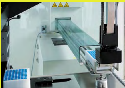
The plate carrier transports samples between the Small-Size Store (SSS) and Freedom EVO
