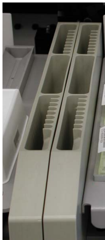
Figure 1b Standard wash stations. The front and rear sections are the deep and shallow wash stations, respectively; the middle section is the waste.
