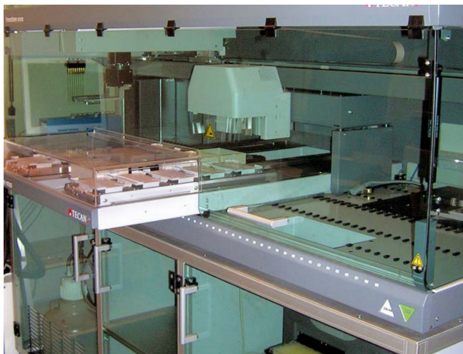
Figure 2: The Freedom EVO system to produce and normalize the genome-wide esiRNA libraries. For UV measurements to determine the RNA concentration, the RoMa arm lifts the plates down from the work table to the GENios Plus reader, which is placed on the level below, as seen in the lower right corner.
